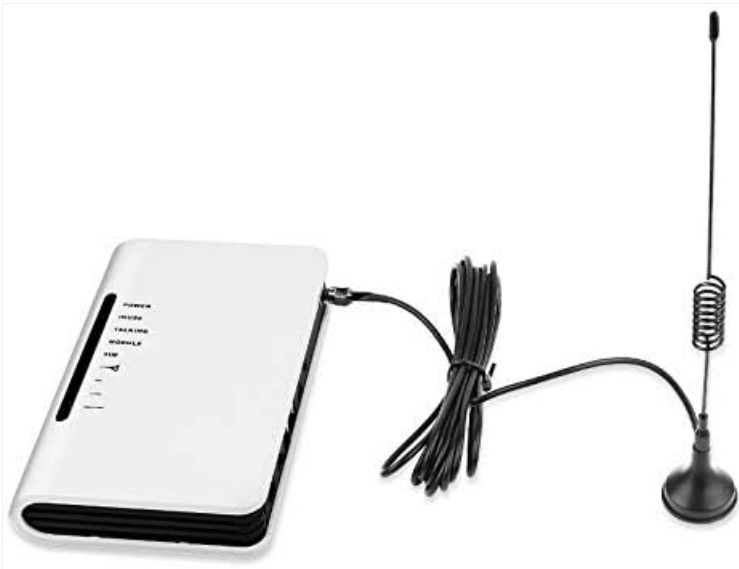
Image: Front view of the Onvian Fixed Wireless Terminal, highlighting the LED indicators for Power, Inuse, Talking, Module, and SIM status.
