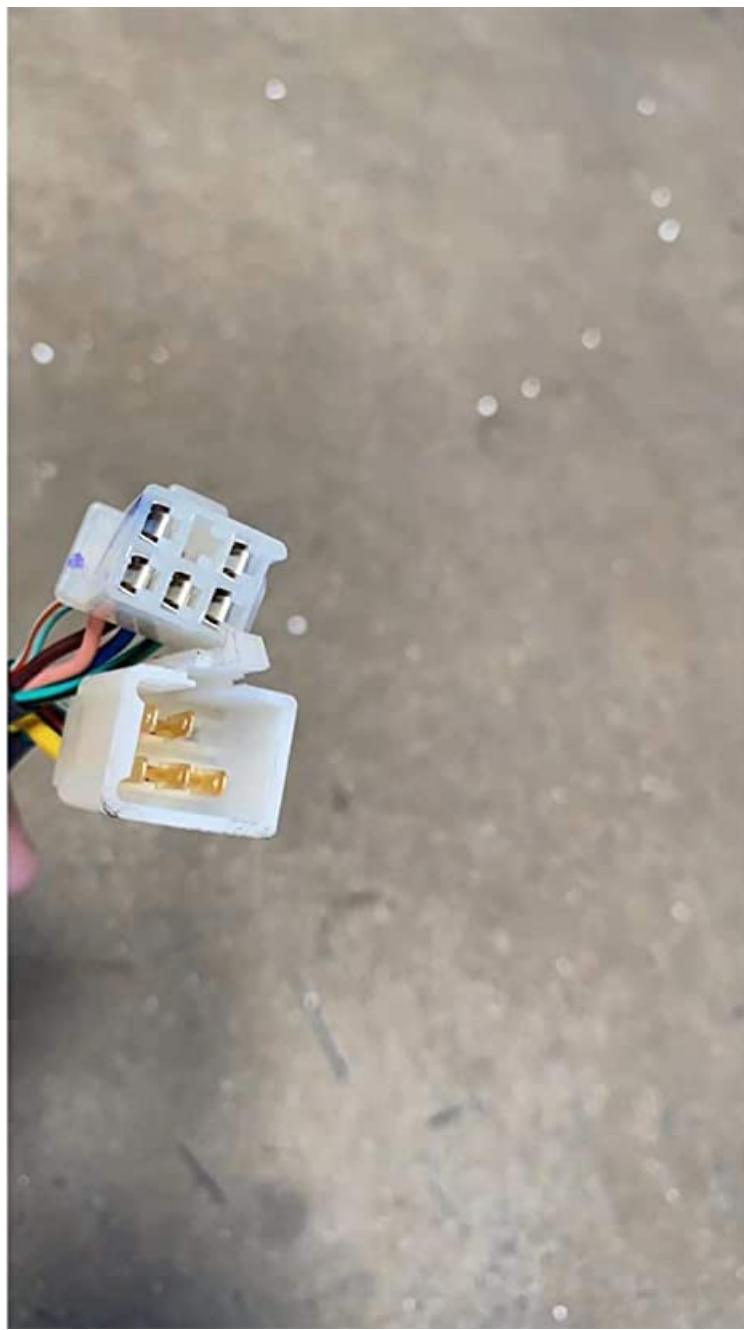
Image 4.1: Close-up of the engine's electrical wiring connector. Ensure compatibility with your bike's harness.
