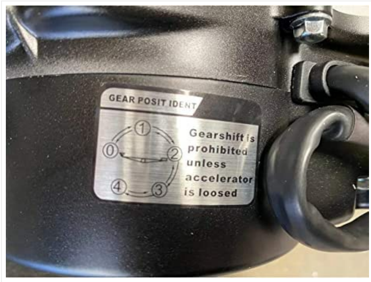
Image 3.1: Gear shift pattern diagram on the engine casing, indicating neutral (0) and gears 1-4. Note: Gearshift is prohibited unless accelerator is loosened.
