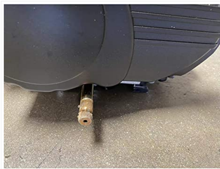
Image 6.1: Location of the engine's oil drain plug for maintenance.
