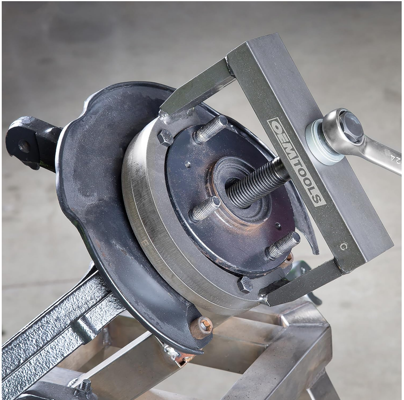
Image: The OEMTOOLS 27213 kit actively removing a wheel hub from a vehicle's knuckle.
