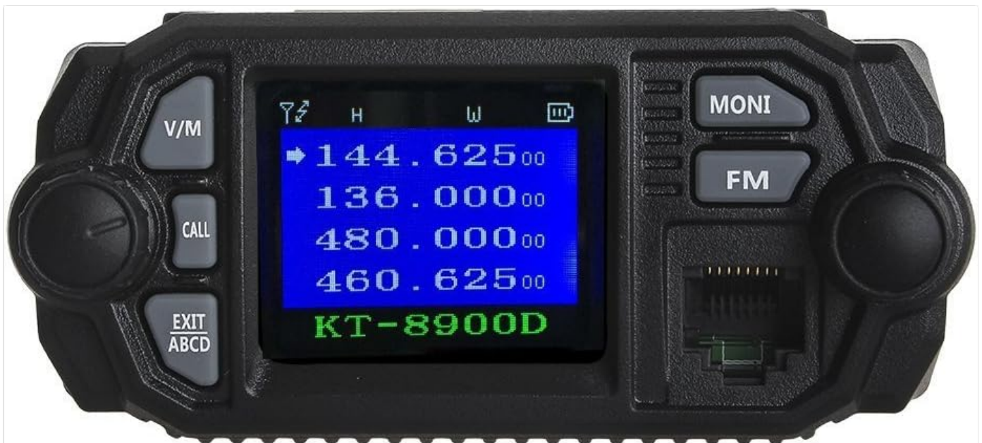
Image: Front view of the QYT KT-8900D showing the LCD display, control knobs, and function buttons.
