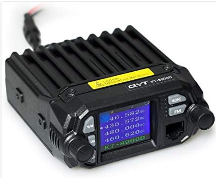
Image: The QYT KT-8900D radio connected to its DC power cable with a cigarette lighter plug for vehicle use.
