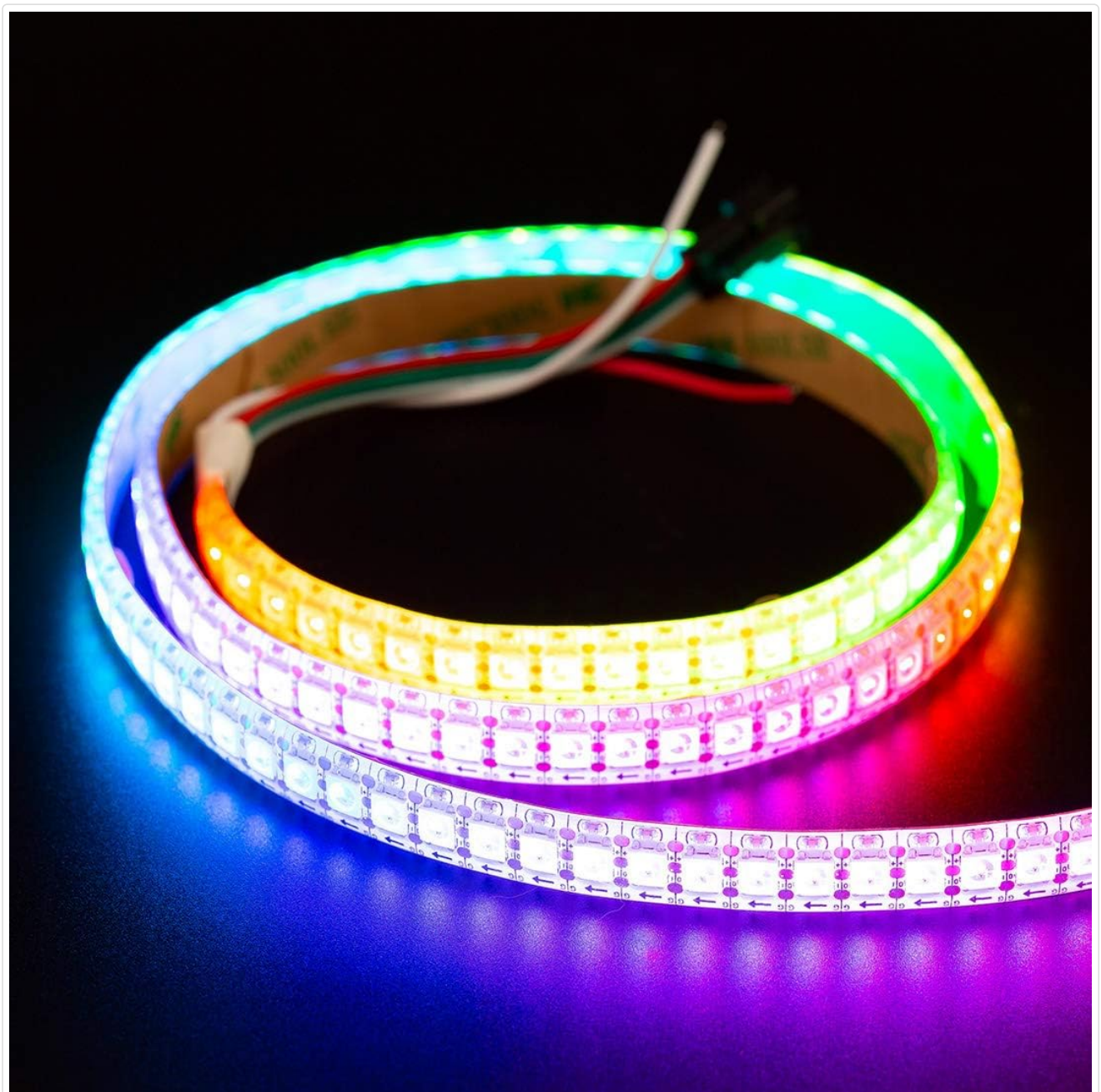
Image: The LED strip illuminated with a vibrant array of colors, demonstrating its individually addressable capabilities.
