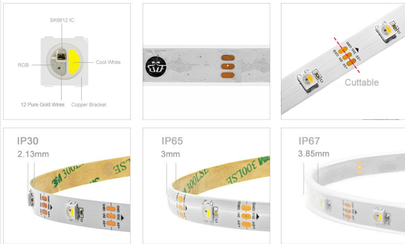
Image: Visual representation of the SK6812 IC, showing where the strip can be cut, and a comparison of IP30, IP65, and IP67 waterproof ratings with their respective thicknesses.
