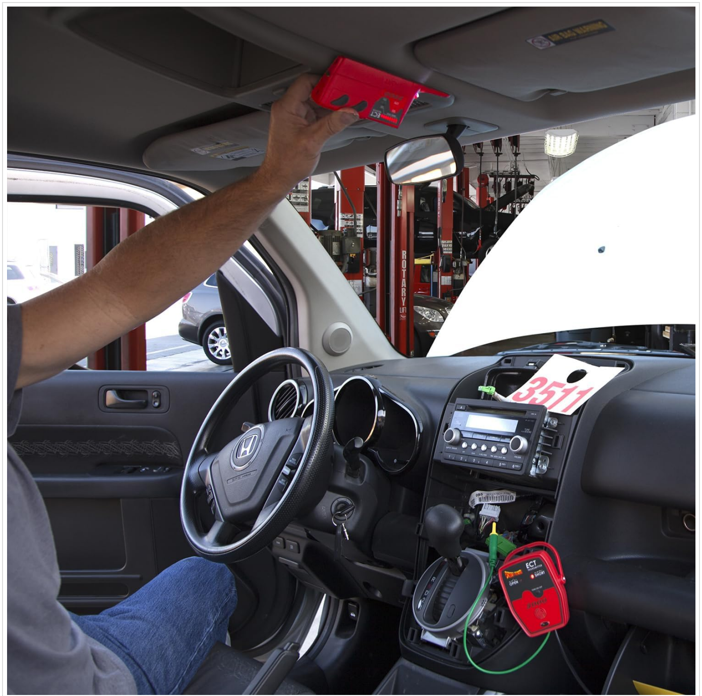
Image: A user is shown tracing a circuit near the headliner of a car using the ECT3000B receiver, illustrating the tool's versatility in reaching various parts of a vehicle's electrical system.
