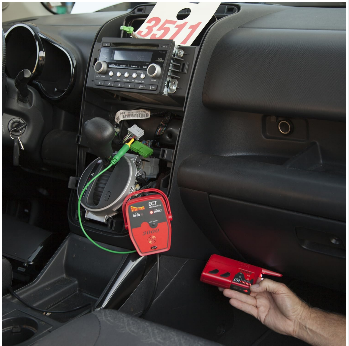
Image: The ECT3000B transmitter is shown connected within the dashboard area of a vehicle, while a user holds the receiver unit, demonstrating its use for tracing electrical circuits in a confined space.
