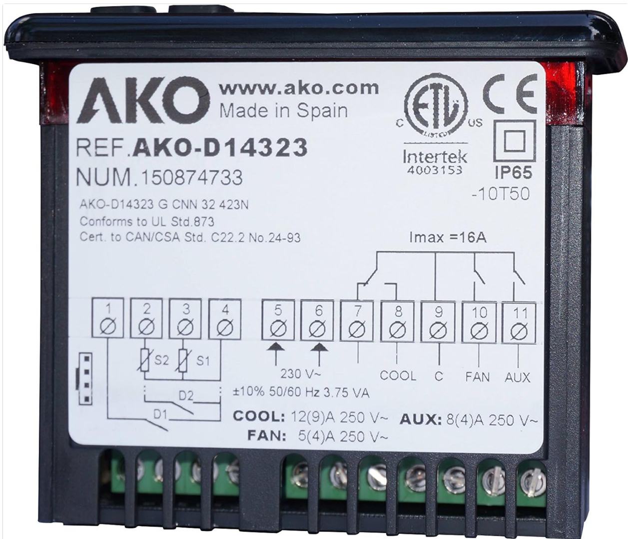
Image 4.1: Back view of the AKO D-14323 controller, displaying the wiring diagram and product specifications. This diagram illustrates connections for power (230V), sensors (S1, S2), compressor (COOL), fan, and auxiliary outputs, along with digital inputs (D1, D2).
