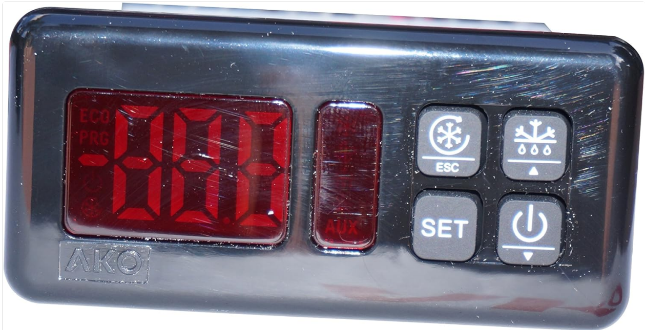
Image 3.1: Front view of the AKO D-14323 controller, showing the digital display and control buttons. The display shows temperature readings, and buttons include ESC, SET, Power, and up/down arrows (often used for defrost and parameter adjustment).
