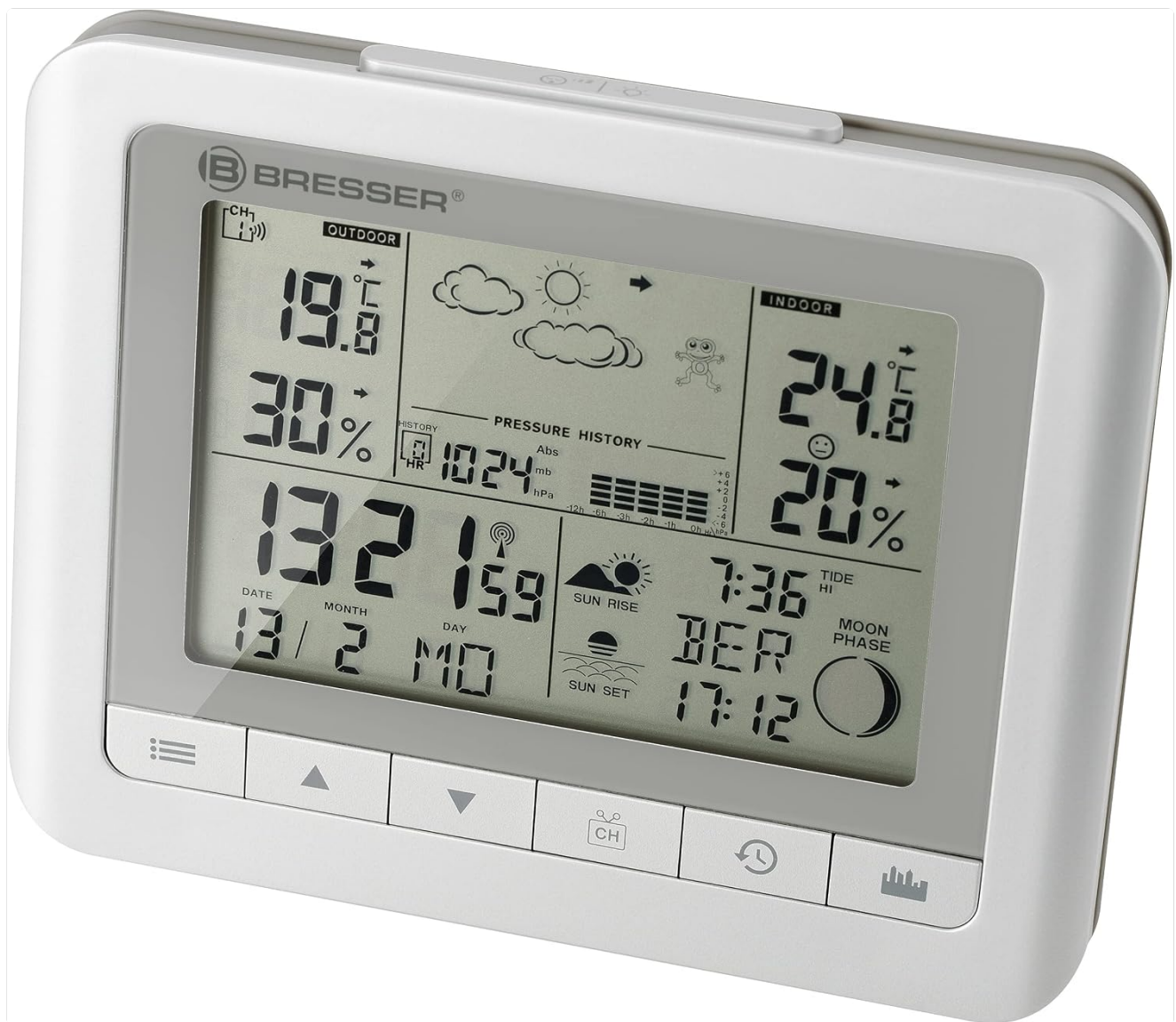
Image 6.1: A detailed view of the main unit's display, showing various weather and time data.
