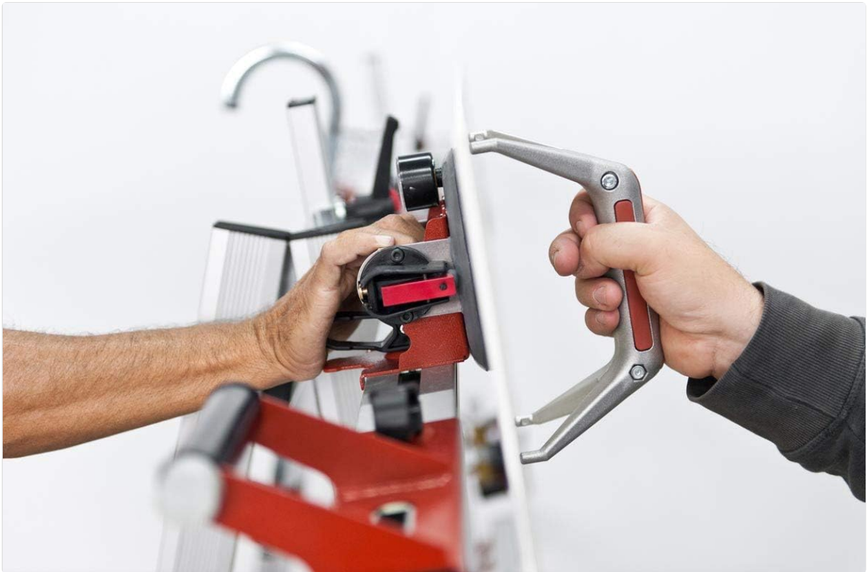
Figure 5: Detail of a hand gripping a suction cup handle, illustrating the secure attachment of the tile to the transport frame.
