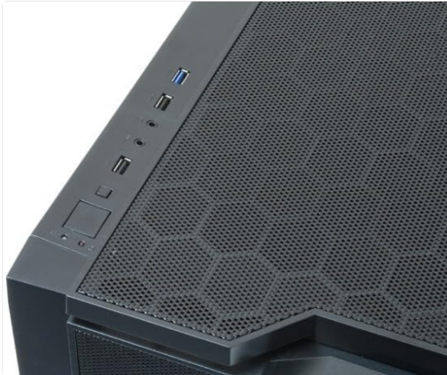
Figure 2: Top panel with front I/O ports.
