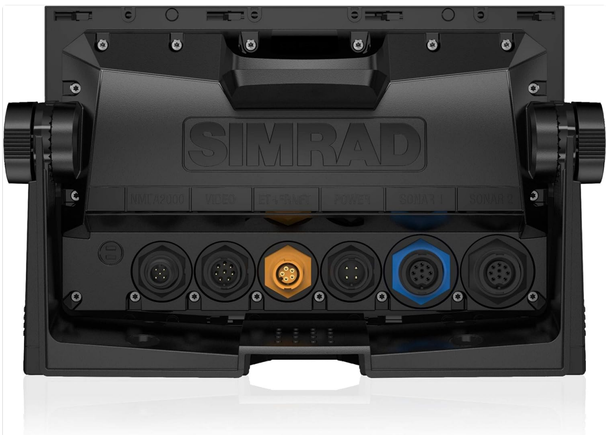
Figure 2.4: Rear view of the Simrad NSS evo3, highlighting the various connectivity ports including NMEA2000, Video, Ethernet, Power, Sonar 1, and Sonar 2.
