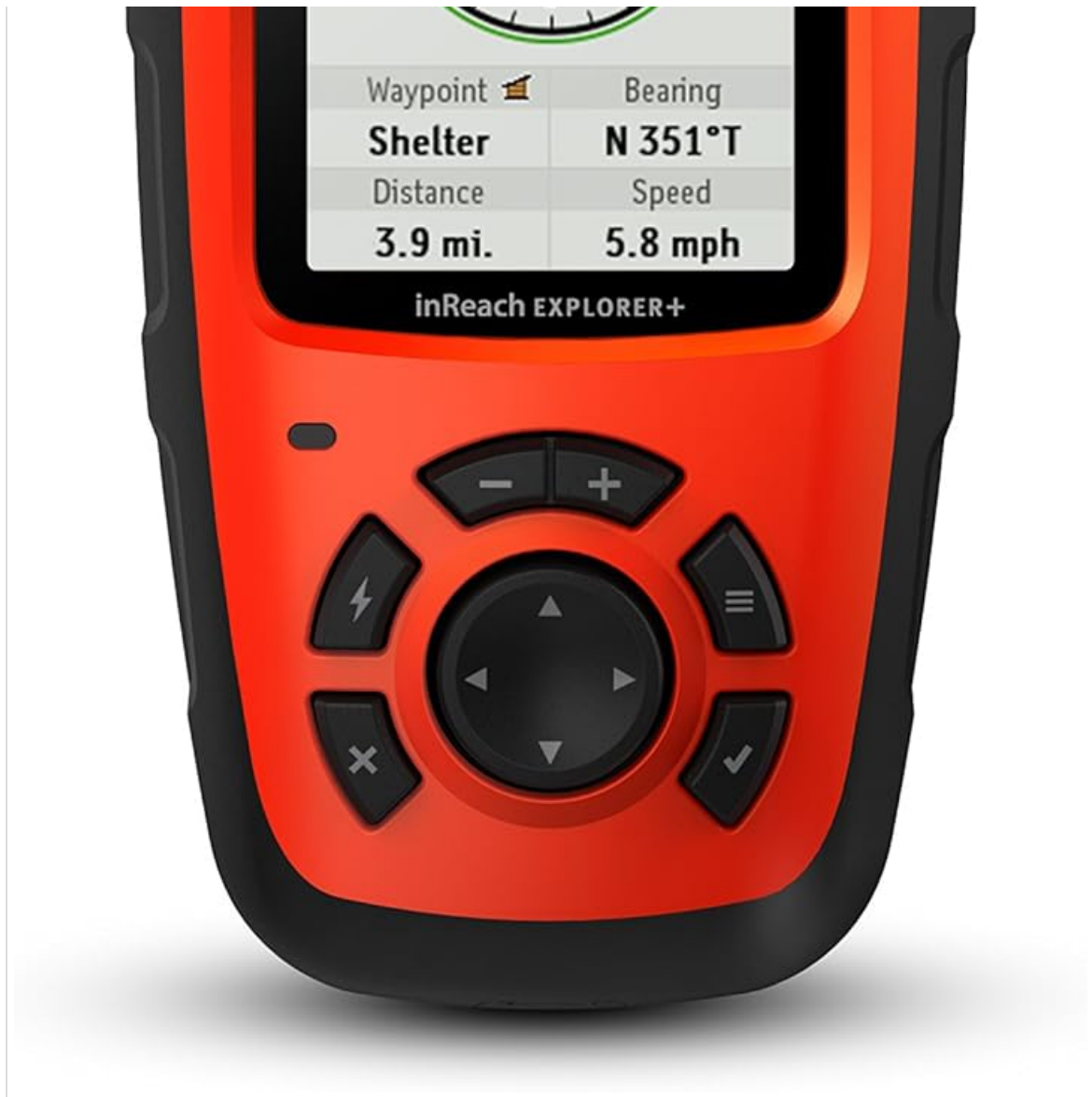
Figure 2: The inReach Explorer+ showing the digital compass and navigation data, including waypoint distance and bearing.
