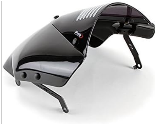
Image 1: Side view showing the screen and its mounting brackets. Note the 'SV' laser-cut into the bracket.
