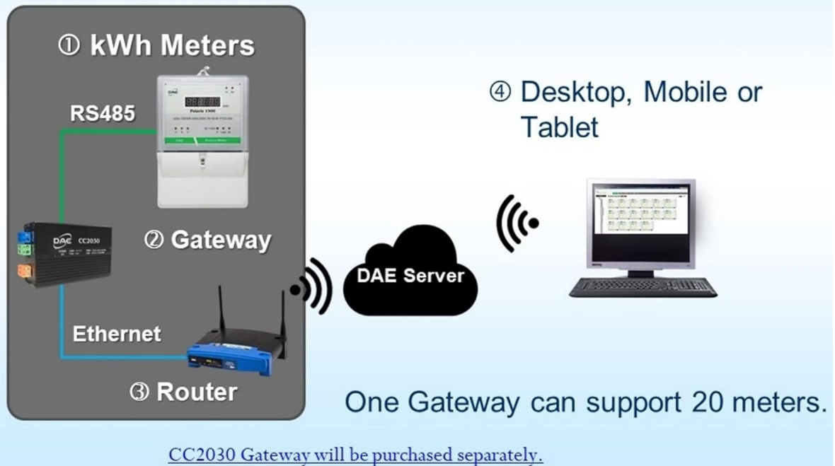
Figure 5: Cloud System Architecture for DAE kWh Meters. The meter connects to a CC2030 Gateway via RS485, which then connects to a router via Ethernet to send data to the DAE Cloud Server.
