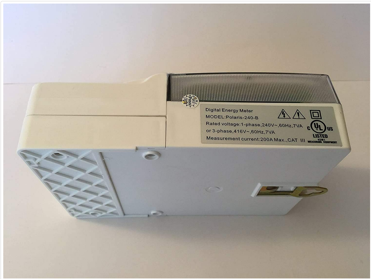
Figure 4: Bottom view of the DAE Digital Energy Meter, showing the product label with model and electrical ratings.
