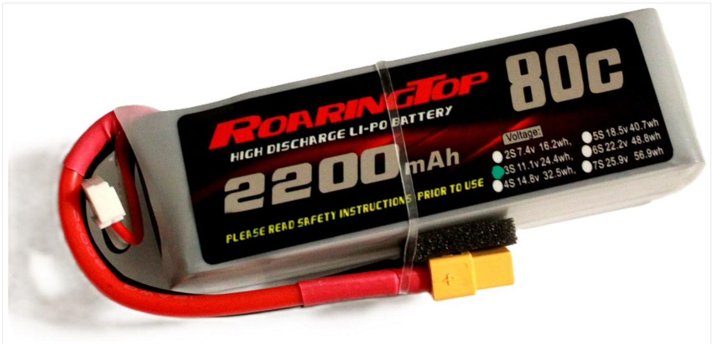
Figure 1: RoaringTop 80C 2200mAh 3S 11.1V LiPo Battery Pack. This image shows the grey battery pack with red wires, an XT60 discharge plug, and a white JST-XH balance plug. The label displays "RoaringTop HIGH DISCHARGE LI-PO BATTERY 2200mAh 80C" and voltage specifications for 2S to 7S configurations.
