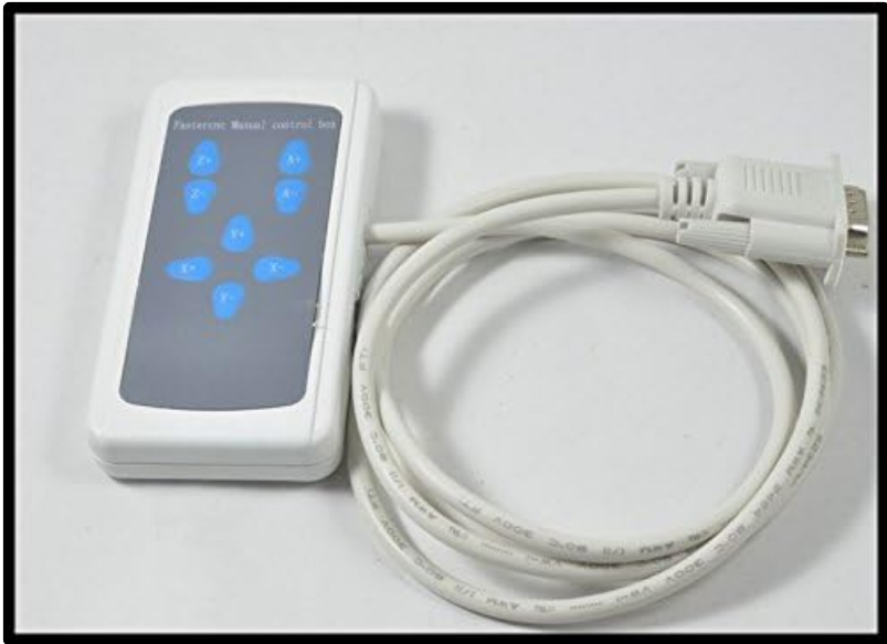
Figure 5: The RS232 Remote Controller for manual, offline operation.
