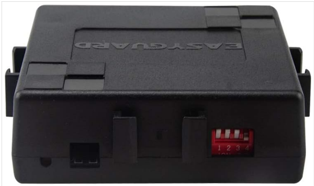
Image 4.1.2: Top view of the main control unit, highlighting the DIP switches (red) for configuration.
