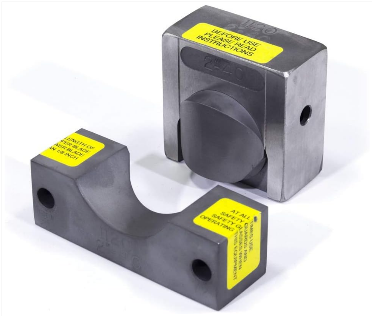
Figure 3.1: Edwards Pipe Notcher Dies (AC1047). This image displays the two primary components of the Edwards Pipe Notcher Dies. The larger, block-shaped die features a curved cutting surface and a label indicating 'BEFORE USE PLEASE READ INSTRUCTIONS'. The smaller, U-shaped die also has a curved surface and labels with safety warnings and an instruction regarding blade length.
