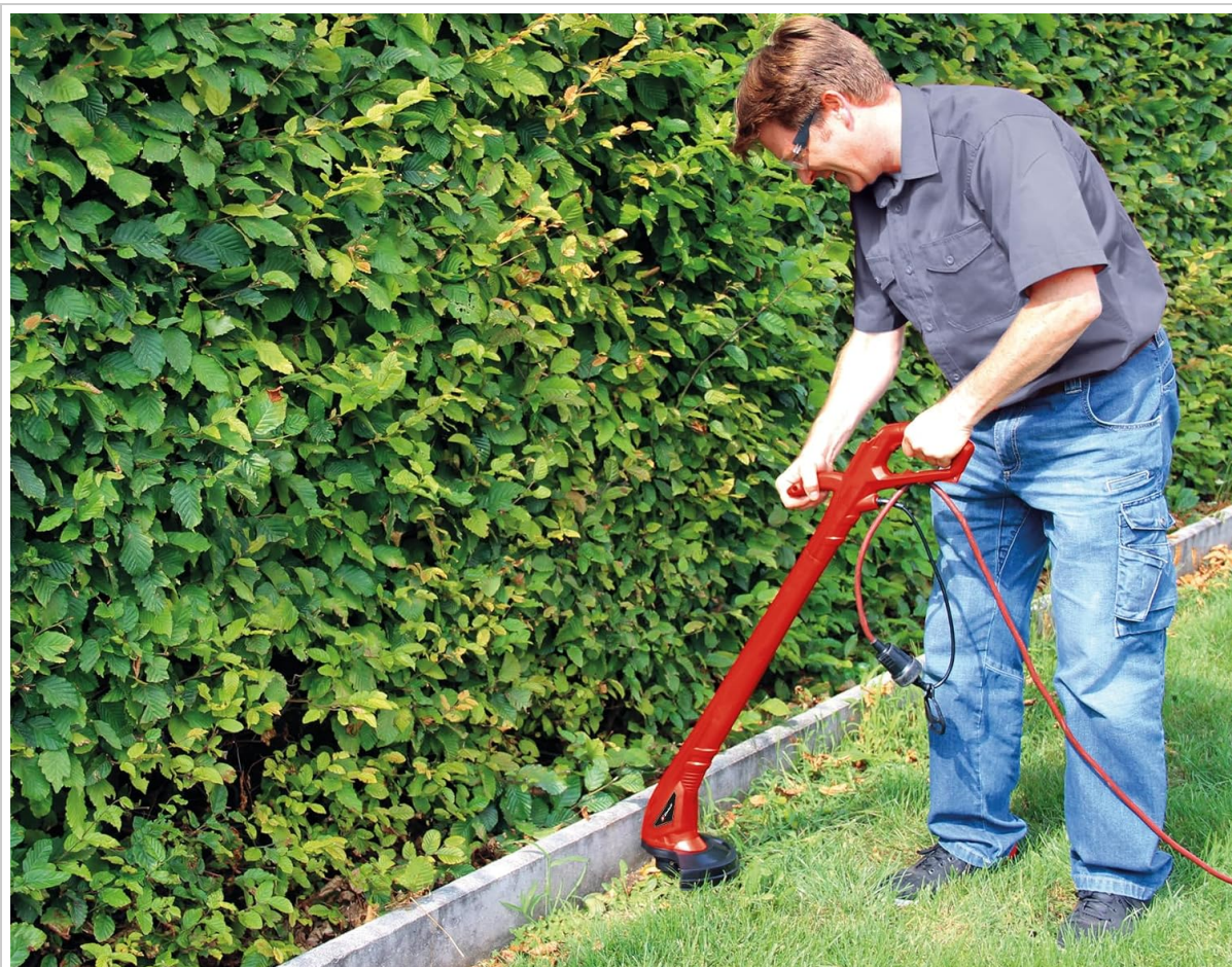
Image 4: A person demonstrating the proper two-hand operation of the Einhell GC-ET 2522 Electric Grass Trimmer for trimming lawn edges.
