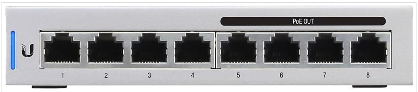
Figure 1: Front Panel of US-8-60W. Ports 1-8 are visible, with "PoE OUT" labeled above ports 5-8. A blue LED indicator is on the left side.
