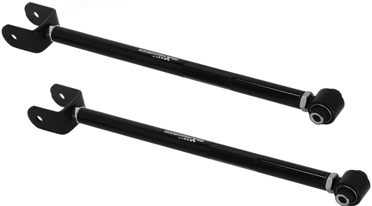
Image 1.1: Overview of the maXpeedingrods Rear Lower Adjustable Camber Arms and product packaging.
