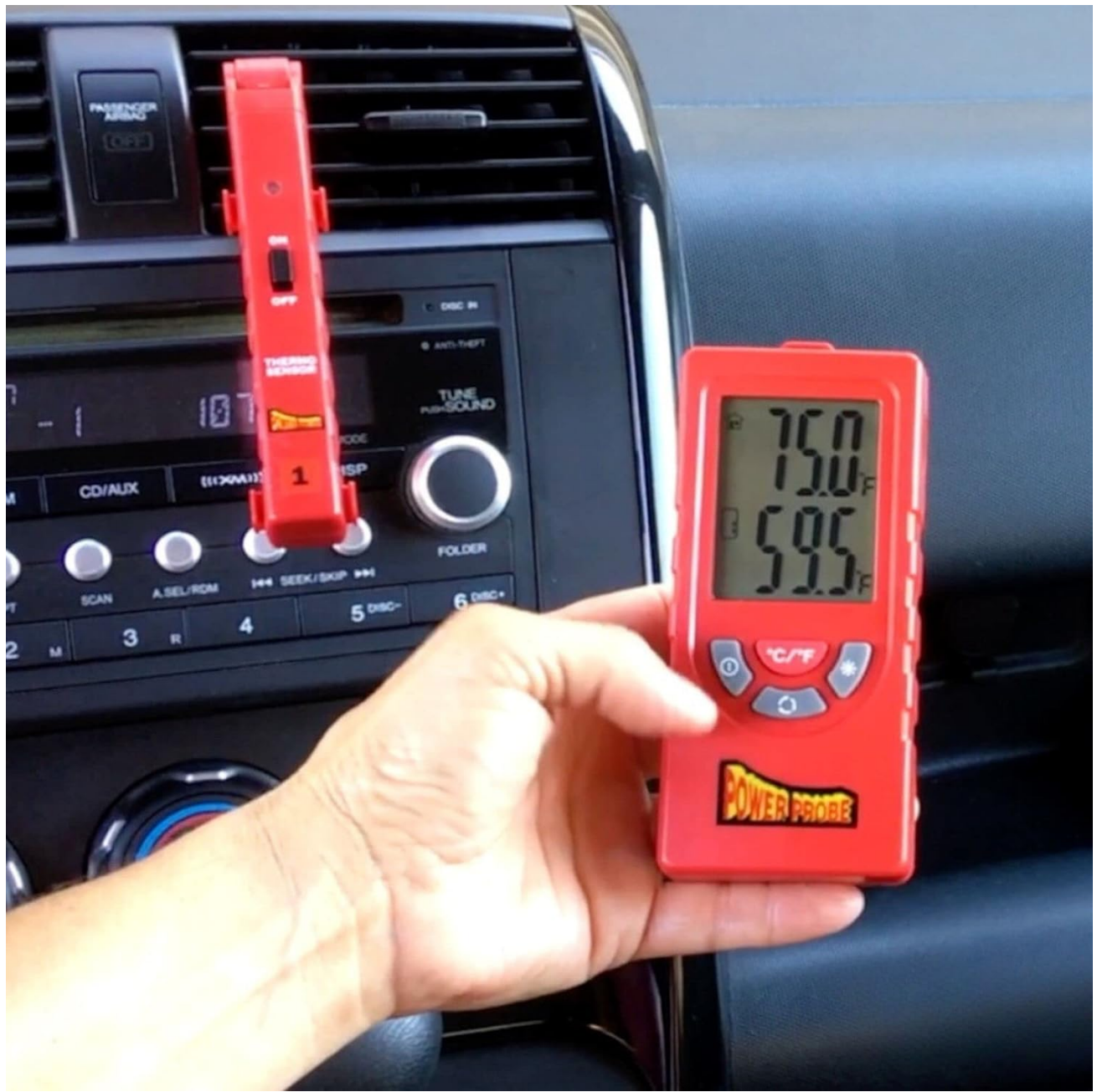
A hand holding the Power Probe TEMPKIT main unit, with a wireless remote sensor clipped into a car's air vent, illustrating the setup for temperature readings.
