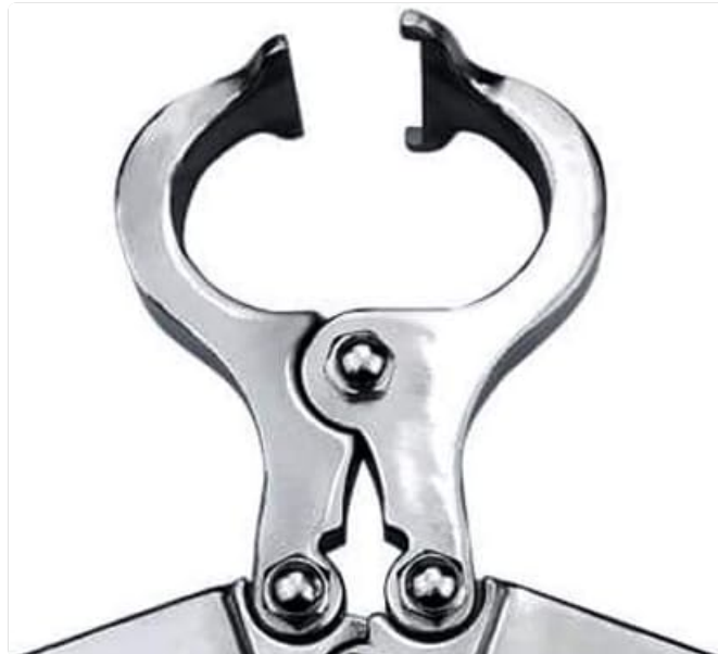
Image 3.1: Close-up view of the plier's jaws, highlighting the crushing mechanism. Ensure these surfaces are clean and free of debris before use.
