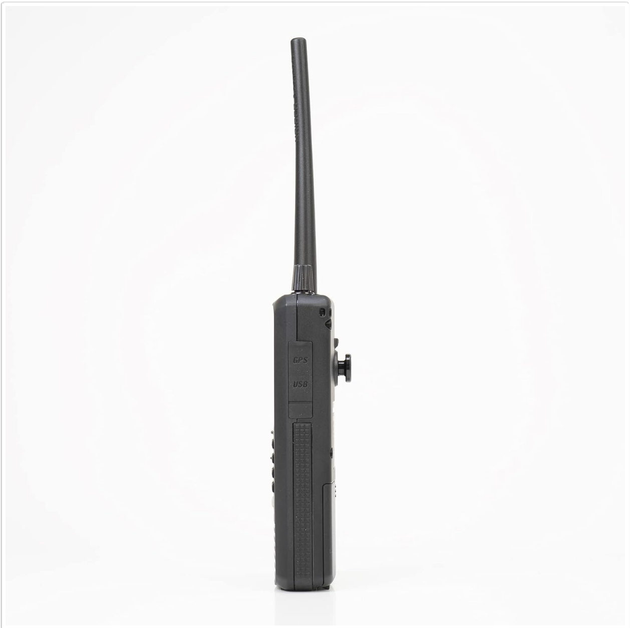
Image: Right side of the scanner, featuring the GPS and USB connection ports.
