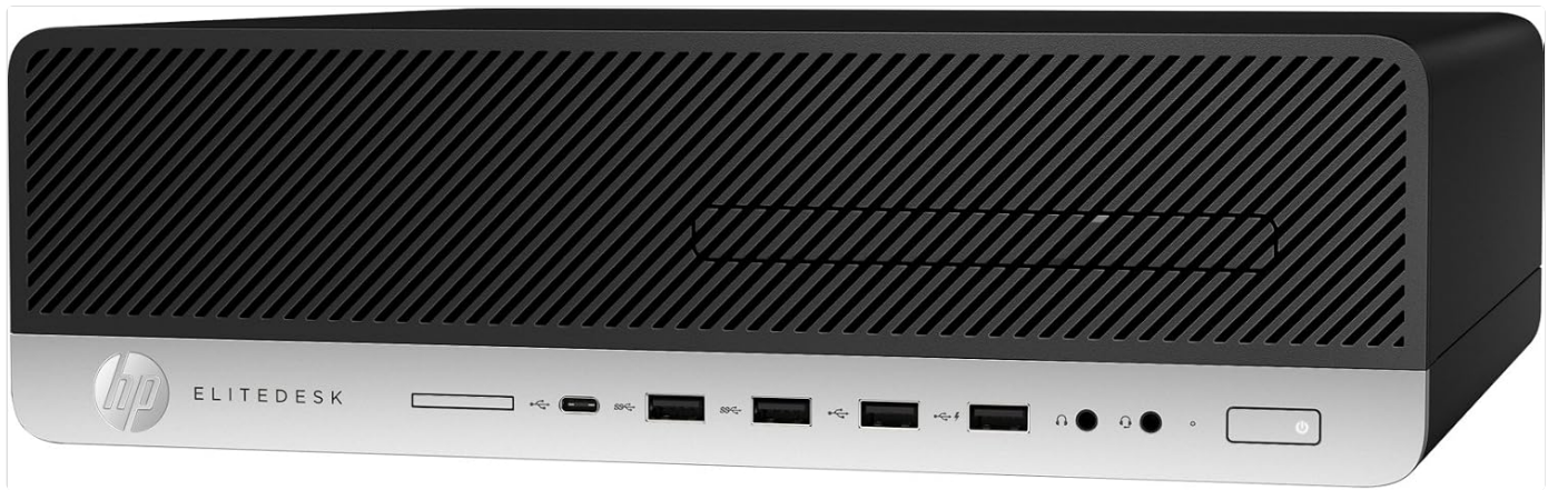
Figure 2.2.1: Front panel of the HP EliteDesk 800 G3 SFF. This view shows the front USB ports (including USB-C), headphone/microphone jacks, and the power button.
