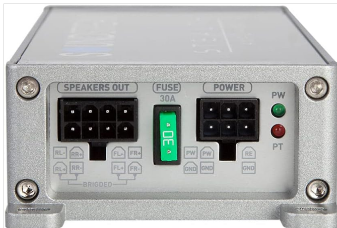
Figure 4.2: Rear panel of the amplifier showing the 'Speakers Out', 'Fuse 30A', and 'Power' terminals. This includes connections for RL-, RR+, FL+, FR- for speakers, and PW, GND, RE for power and remote turn-on.
