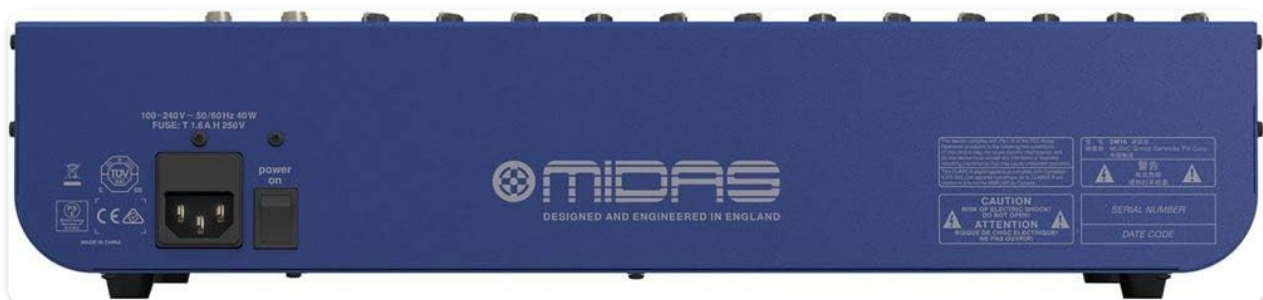
Figure 2.1: Rear panel of the MIDAS DM16 showing power input and warnings.
