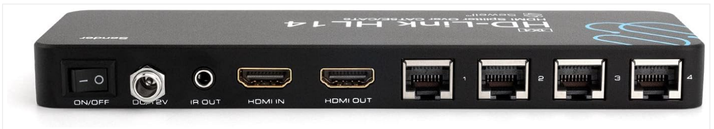
Image: Rear view of the HD-Link HL14 Sender unit, showing the ON/OFF switch, DC 12V power input, IR OUT port, HDMI IN port, HDMI OUT (loop-through) port, and four RJ45 CAT outputs (1-4).
