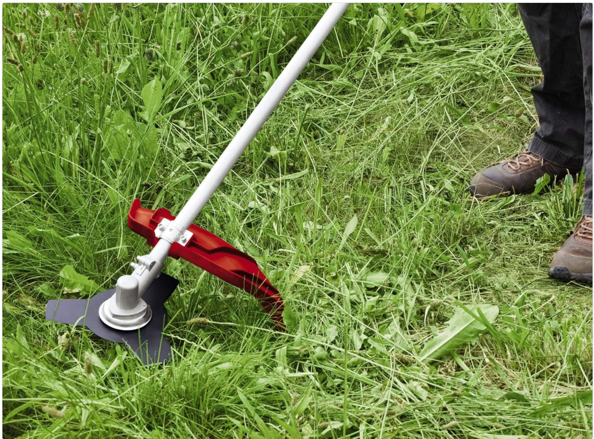
Image: The brush cutter in action, using the 3-tooth blade attachment to clear dense, tall grass.
