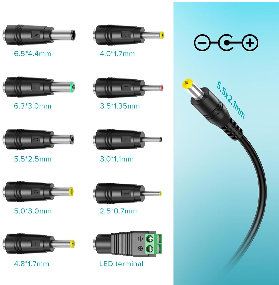
Image: A visual guide displaying ten different DC connector tips with their corresponding dimensions (e.g., 6.5*4.4mm, 5.5*2.1mm). An illustration of a DC plug also indicates the central positive (+) and outer negative (-) polarity.
