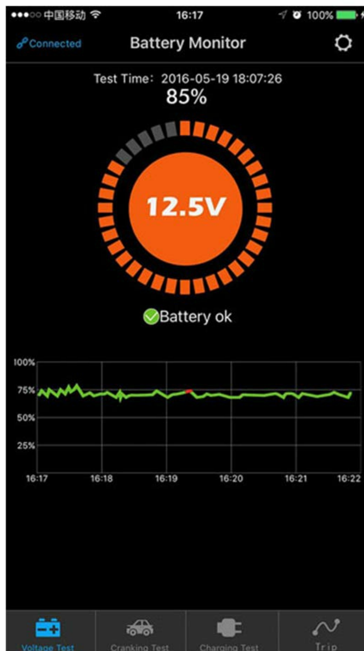
Figure 5.2: Screenshot of the Quicklynks BM2 mobile application displaying real-time battery voltage, State of Charge (SOC), temperature, and a historical voltage graph under the Voltage Test section.
