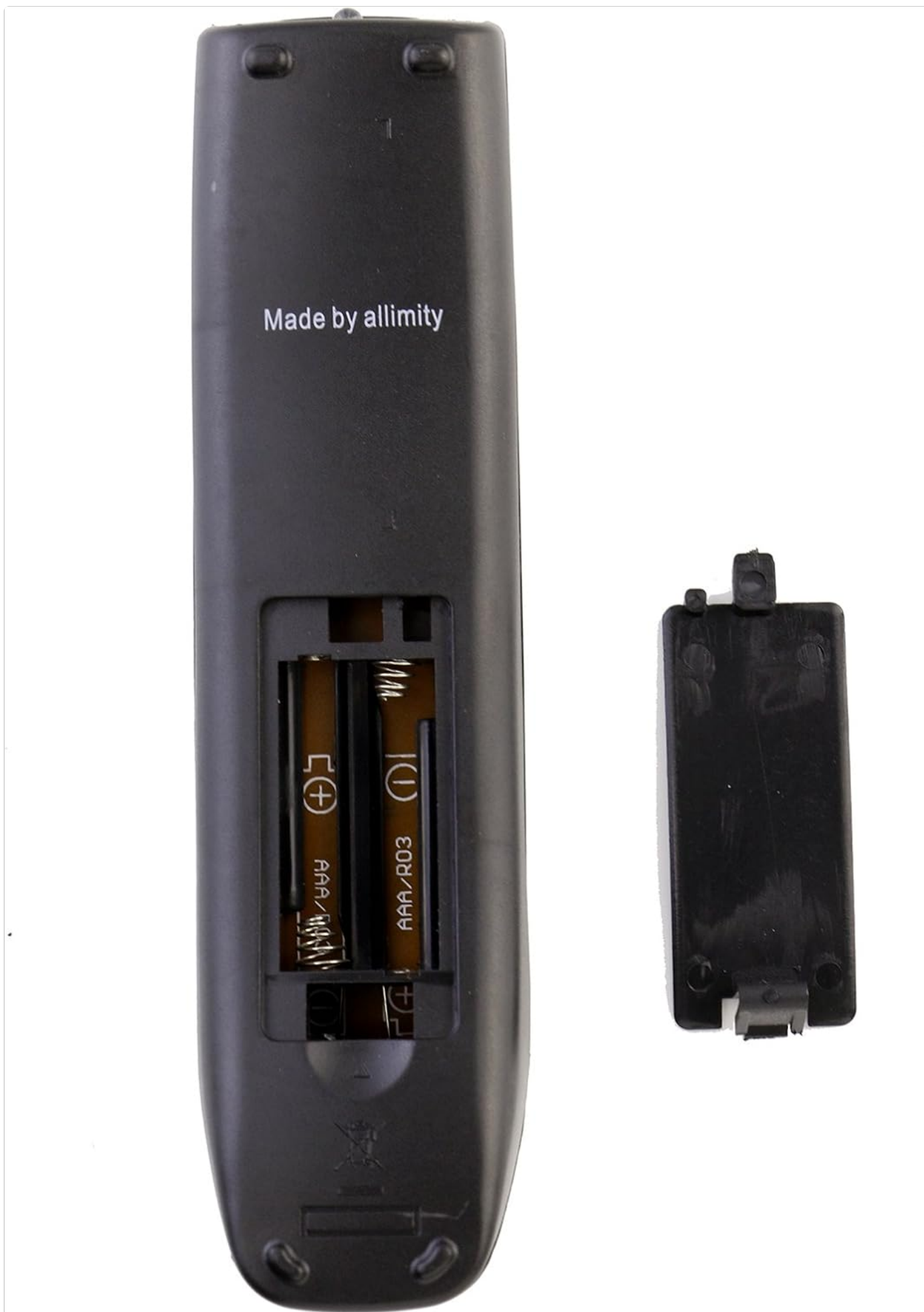
Image: Back of the remote control with the battery compartment open. This image illustrates where to insert the two AAA batteries, showing the correct positive and negative terminal orientation.
