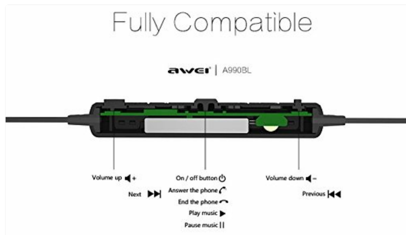
Image 4.4: Inline control button functions. This diagram details the functions of each button on the inline control: Volume Up (+), Volume Down (-), Next Track, Previous Track, and the multi-function button for Power On/Off, Answer/End Call, and Play/Pause Music.
