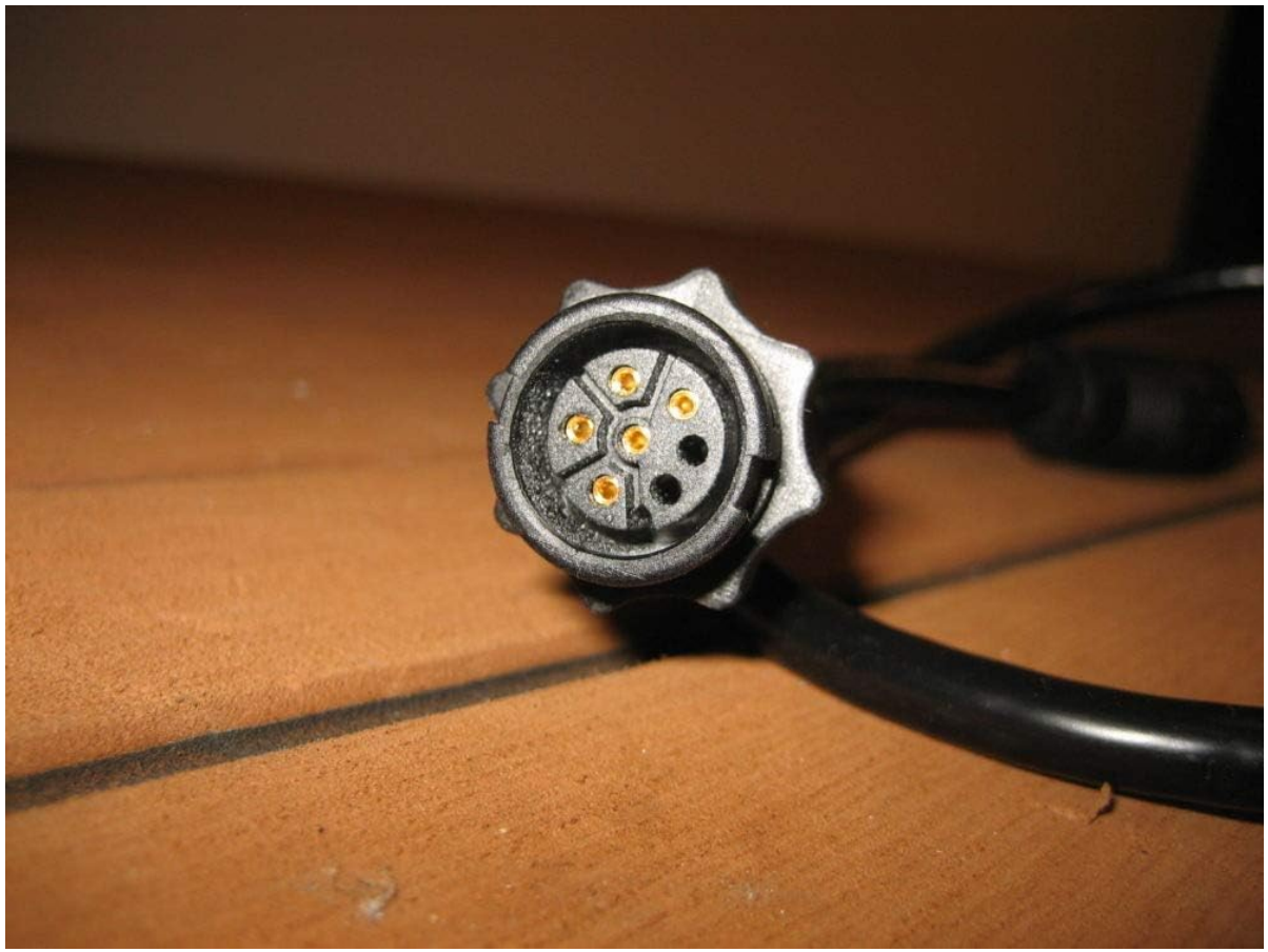
Image 2: Close-up view of the 9-pin connector end of the Lowrance adapter cable, designed to plug into compatible Lowrance fish finders or chartplotters.
