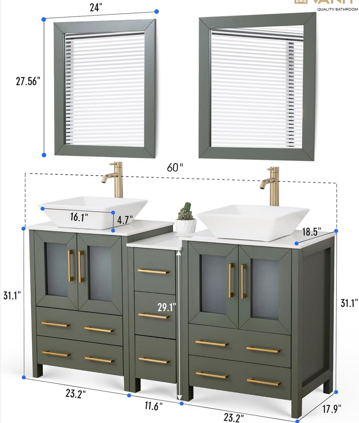
Image 4.1: Dimensions of the vanity and mirrors for installation planning.
