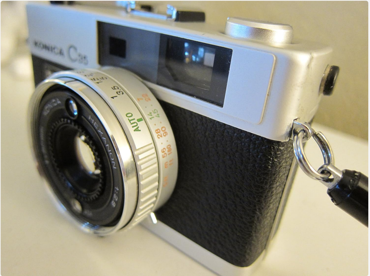
Figure 3: Side view of the Konica C35 camera, highlighting the focus ring with distance markings in meters and feet.
