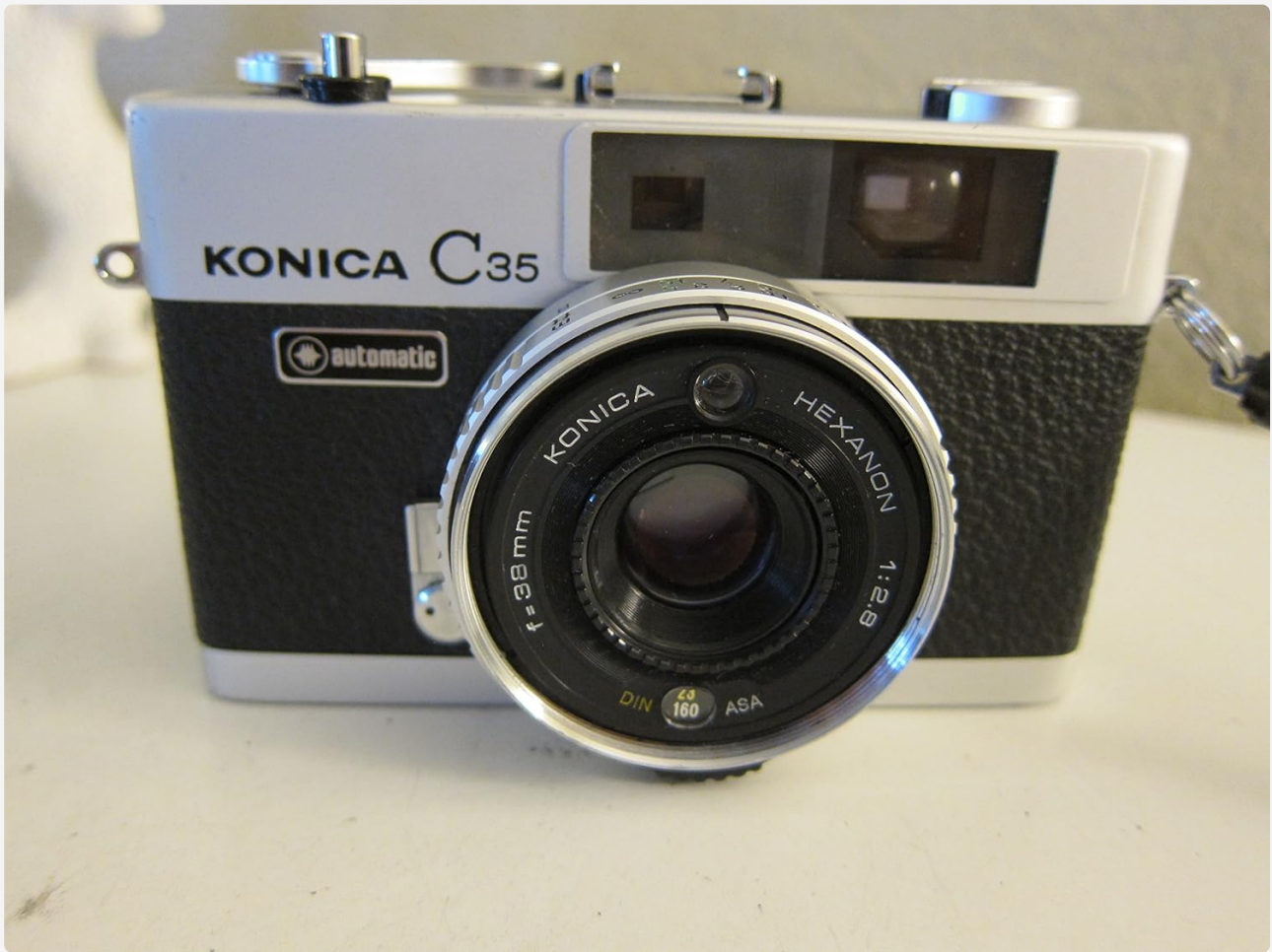
Figure 1: Front view of the Konica C35 camera, showing the Konica Hexanon 38mm F2.8 lens, viewfinder, and "automatic" badge.
