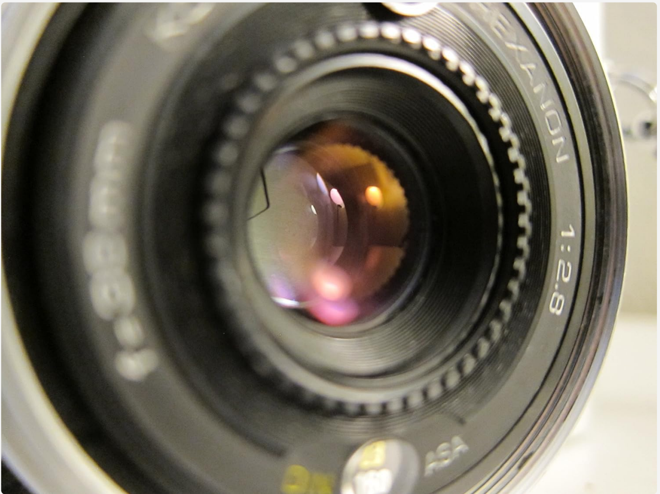
Figure 2: Close-up of the Konic Hexanon 38mm F2.8 lens, showing aperture blades and lens coatings.
