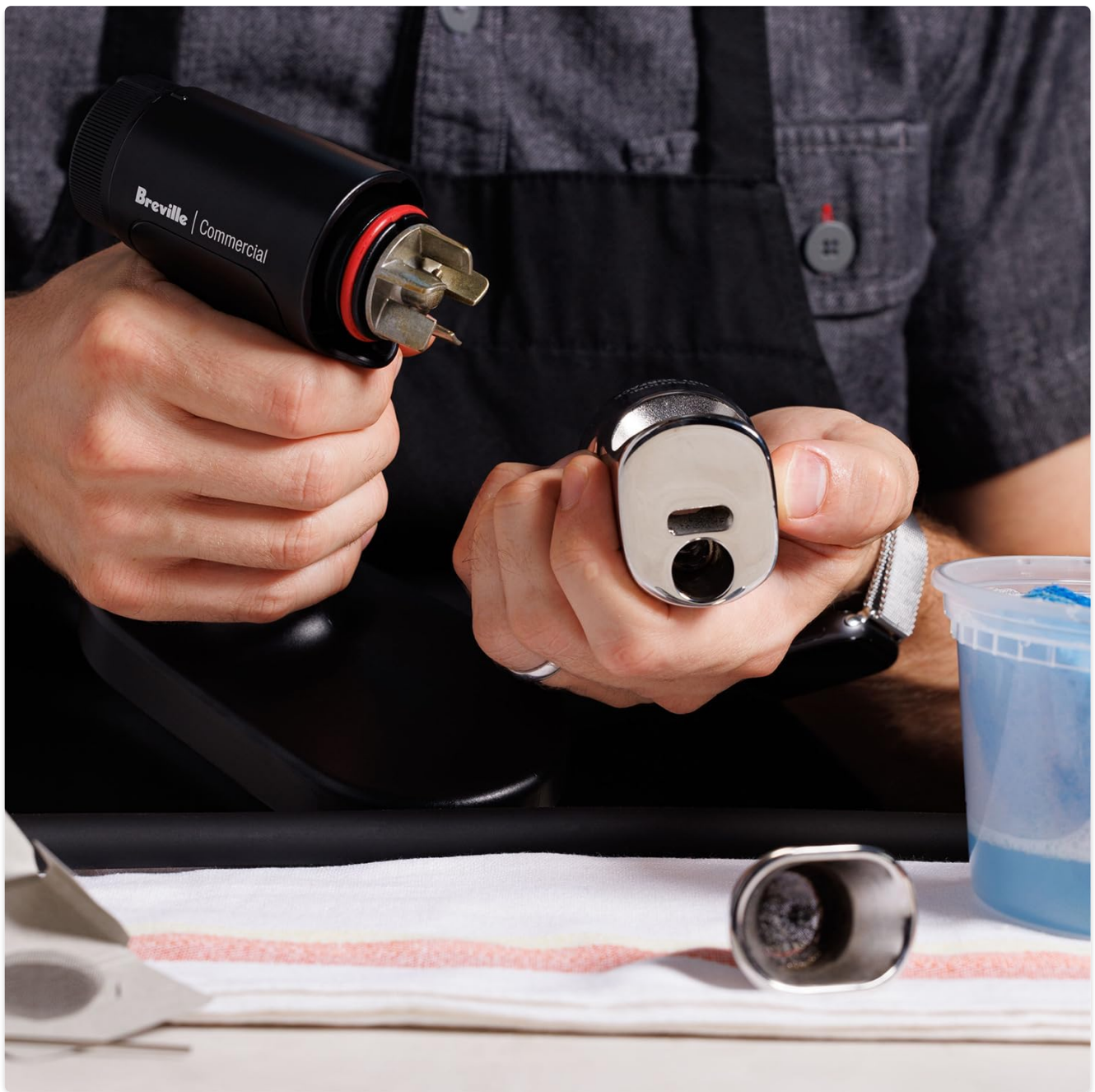
Image: A user demonstrating how to disassemble the burn chamber from the main unit, which is also relevant for initial setup and loading smoking material.
