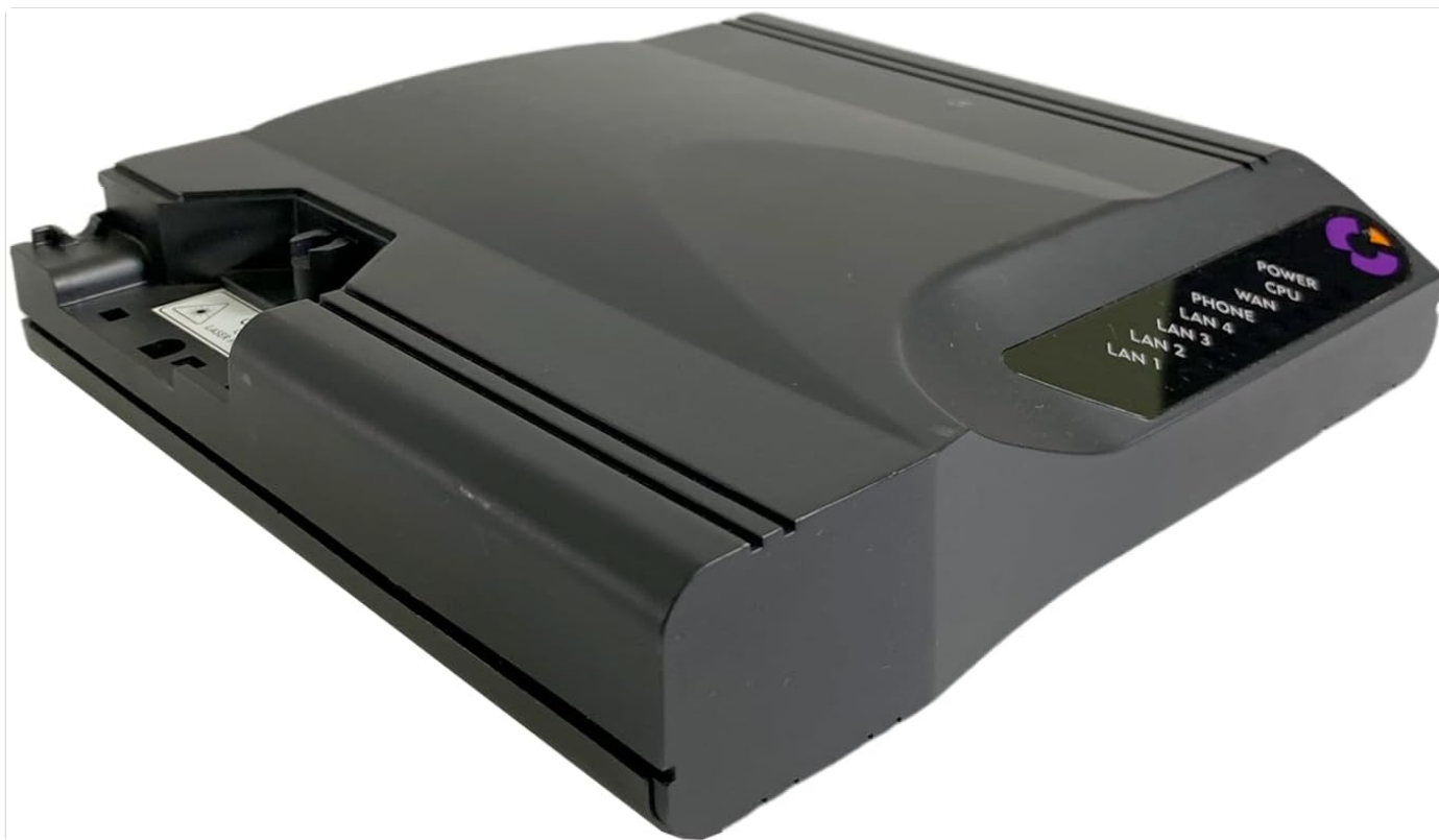
Figure 1: Front and side view of the Calix 716GE-I ONT, highlighting the indicator lights for Power, CPU, WAN, Phone, and LAN ports.
