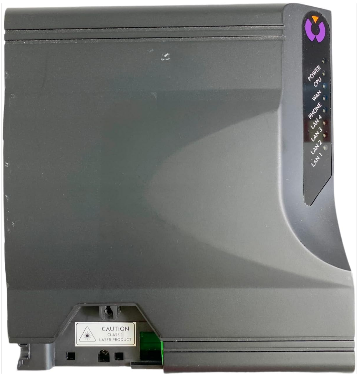
Figure 2: Top view of the Calix 716GE-I ONT, showing the indicator lights and a caution label for Class 1 Laser Product near the fiber input.
