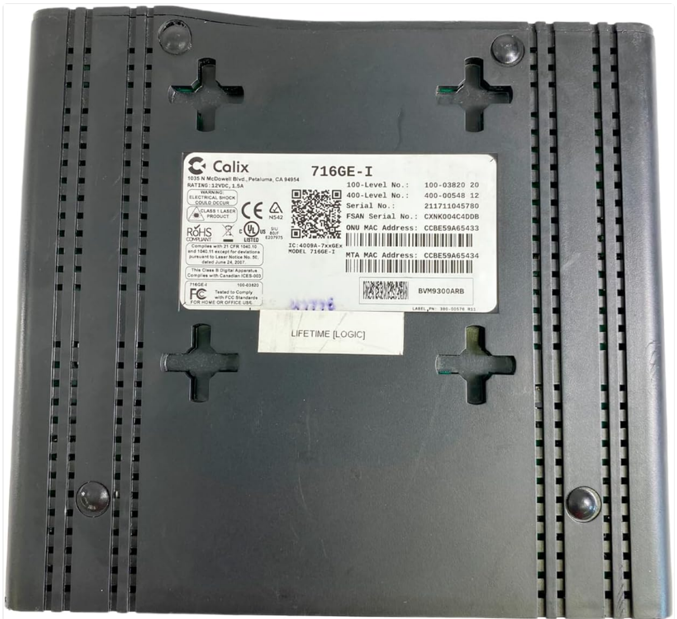
Figure 5: Bottom view of the Calix 716GE-I ONT, showing the product label with model number, serial number, MAC address, and regulatory compliance information. This information is crucial for support and device registration. For more product details, visit: Calix Product Information .
