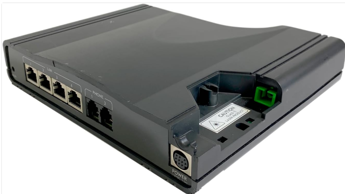
Figure 4: Rear-side view of the Calix 716GE-I ONT, providing a clearer look at the port layout and the fiber optic connection area, which is typically covered or managed by a service technician.
