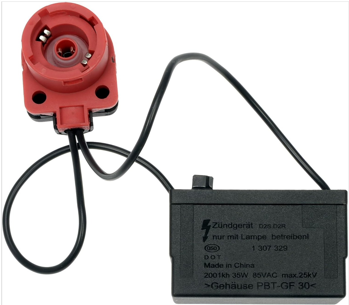
Figure 4.1: Rear view of the Dorman 601-165 igniter, showing the bulb connection point and product labeling. The label indicates compatibility with D2S/D2R bulbs and specifies electrical parameters.
