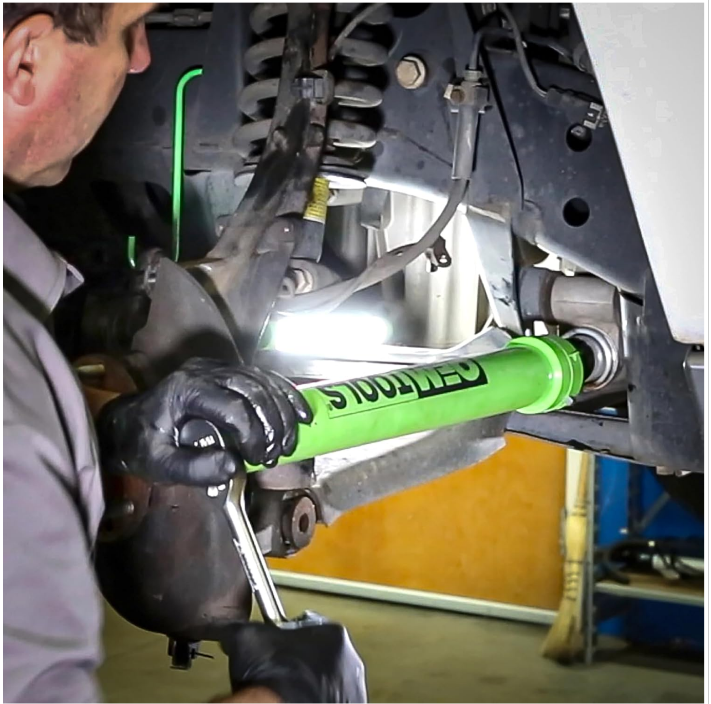
Figure 5: A mechanic demonstrating the use of the OEMTOOLS inner tie rod removal tool to access and work on an inner tie rod within a vehicle's wheel well.
