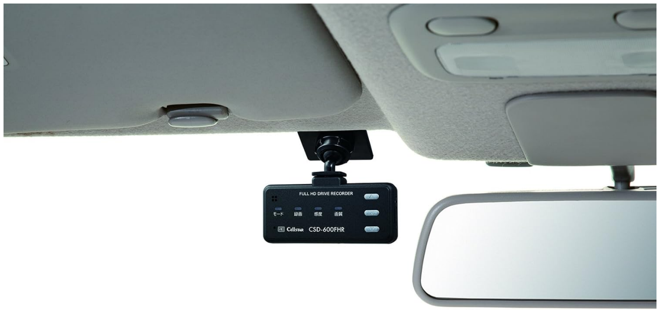
Figure 4.1: Windshield Mounting Example
