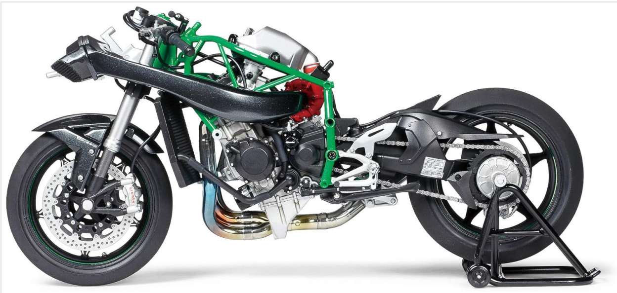
Image: Side view of the model's chassis, showing the green frame, engine, and suspension components.
