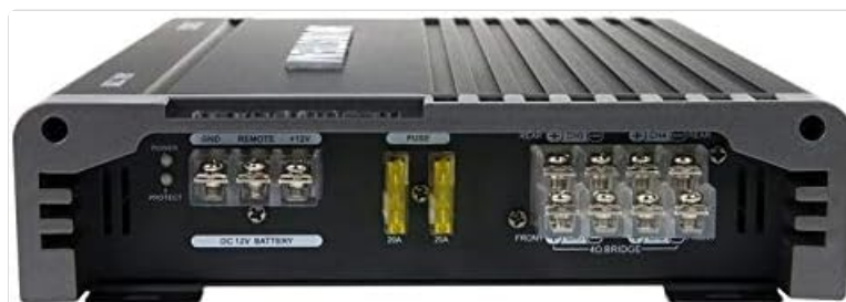
Figure 3: Power and Speaker Terminal Side of AR4.1200 Amplifier. This image shows the connection terminals for power (GND, REMOTE, +12V), dual fuses, and the speaker output terminals for channels 1 through 4, along with bridging options.
