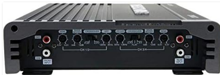
Figure 2: Control Panel of AR4.1200 Amplifier. This image highlights the input and control side of the amplifier, featuring RCA inputs, gain controls, crossover frequency adjustments (HPF and LPF), and bass boost knobs for channels 1/2 and 3/4.
