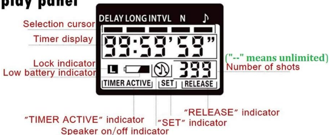
Image 2: Labeled diagram of the PHOLSY C8 Timer Remote Control.
