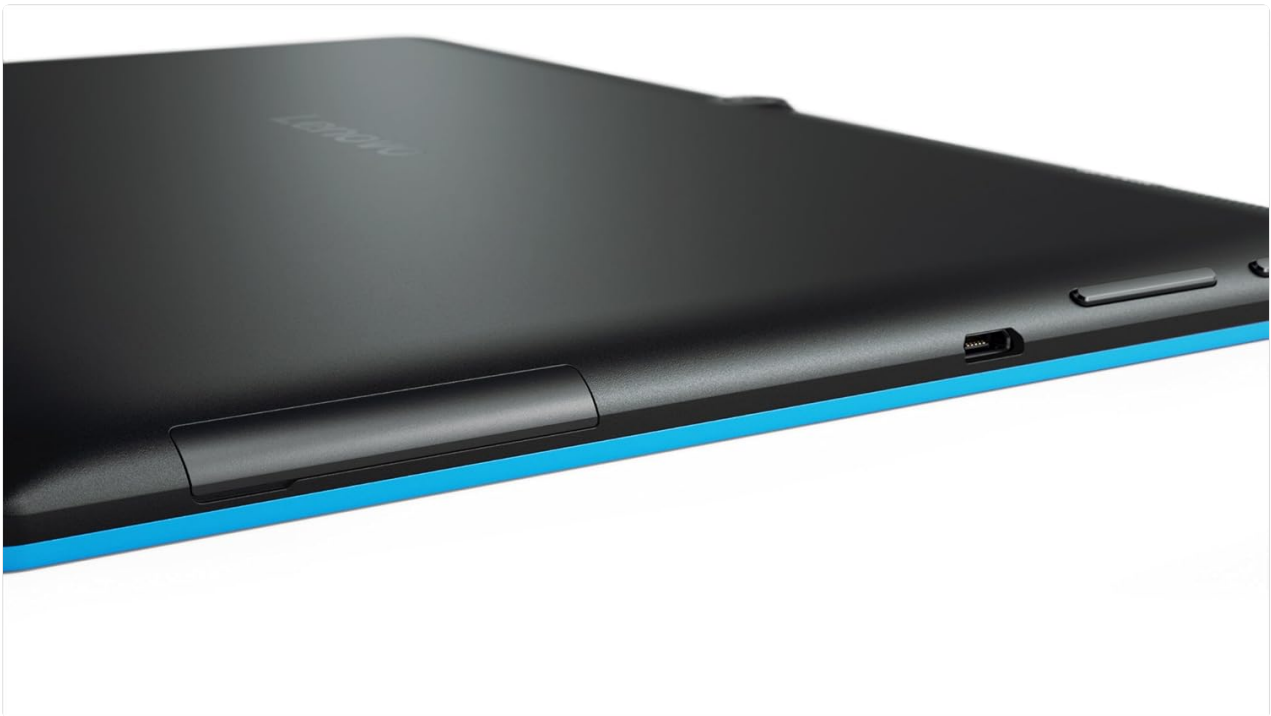
Figure 2: Micro-USB charging port and microSD card slot.
