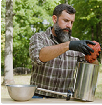
Image: A person loading ground meat into the removable cylinder of the sausage stuffer.
