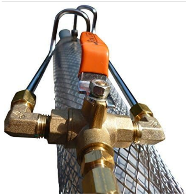
Figure 4: Close-up of the solution valve, which controls the flow of the chosen chemical into the fogging mechanism.
