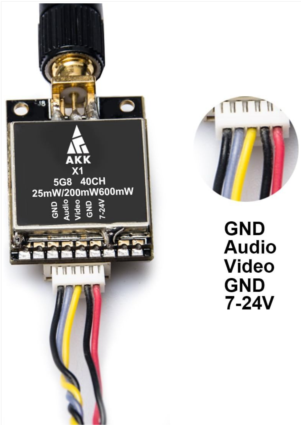
Figure 5.1: Detailed wiring diagram for the AKK X1, illustrating the correct pin connections for power, video, and audio.
