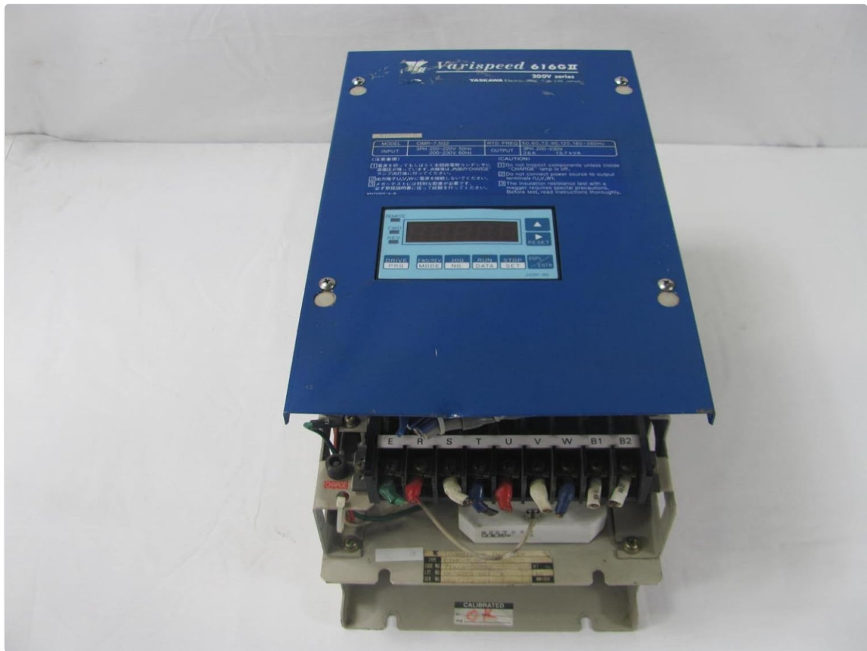
Figure 3: Close-up view of the Yaskawa CIMR-7.5G2 control panel.
