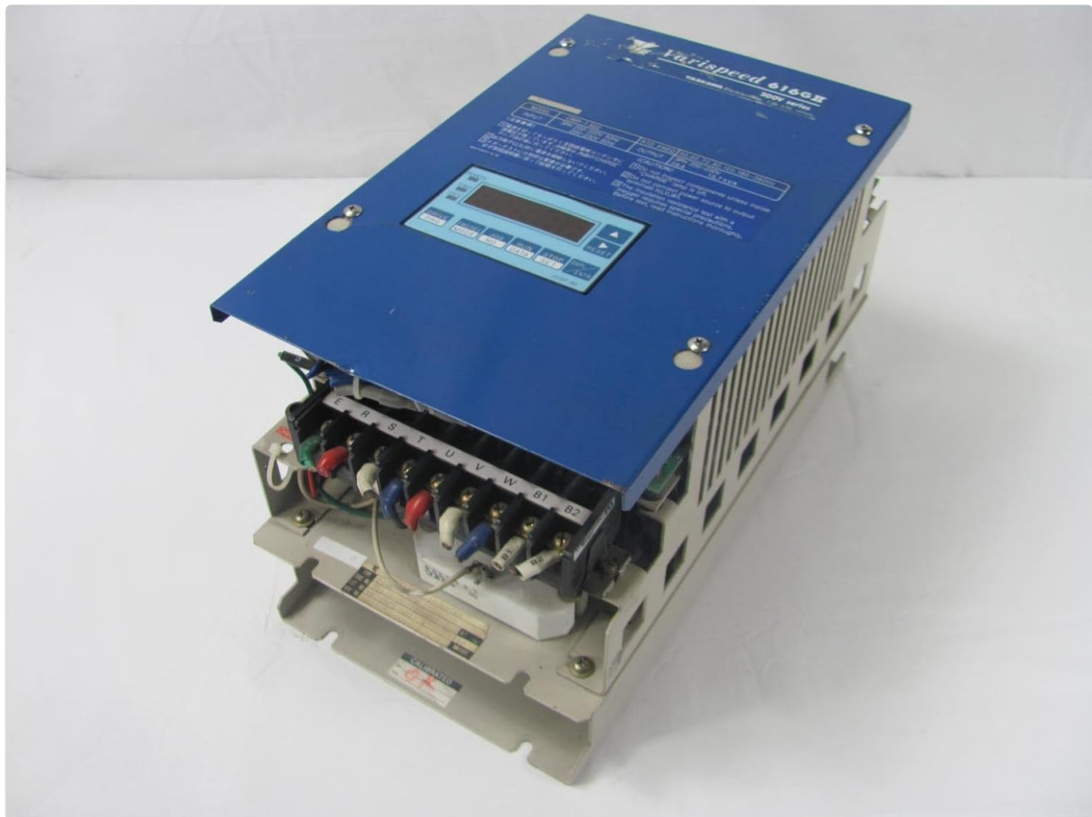
Figure 1: Yaskawa CIMR-7.5G2 Variable Frequency Drive with top cover open, revealing internal components and wiring terminals.
