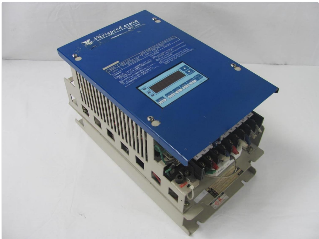
Figure 2: Yaskawa CIMR-7.5G2 wiring terminals for power and motor connections.
