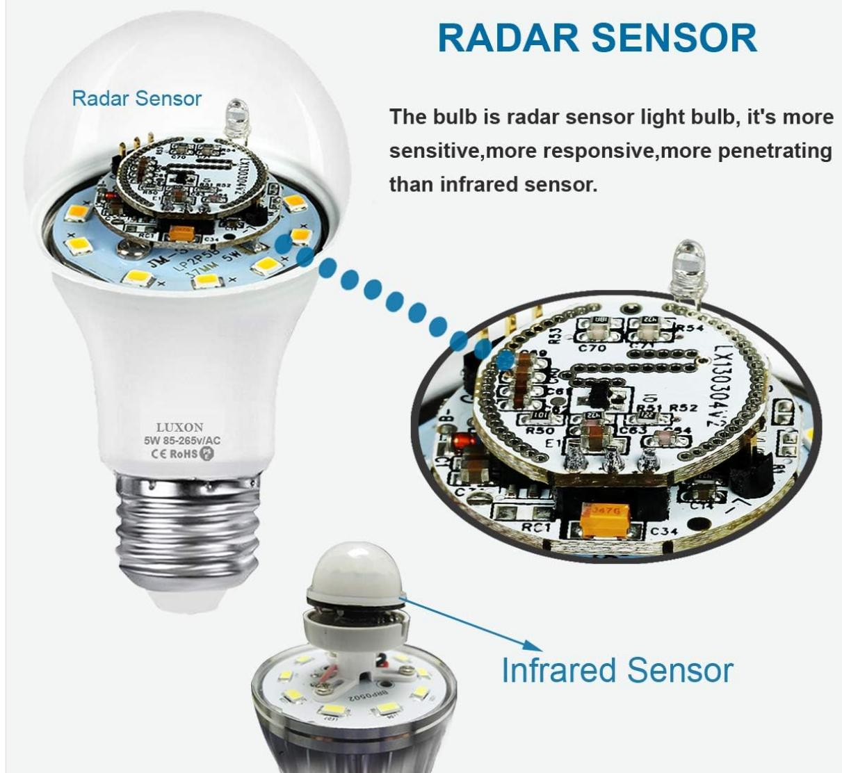
This image illustrates the internal components of the LUXON Radar Sensor LED bulb, highlighting the radar sensor module compared to a typical infrared sensor. The radar sensor is designed for enhanced sensitivity and penetration.
